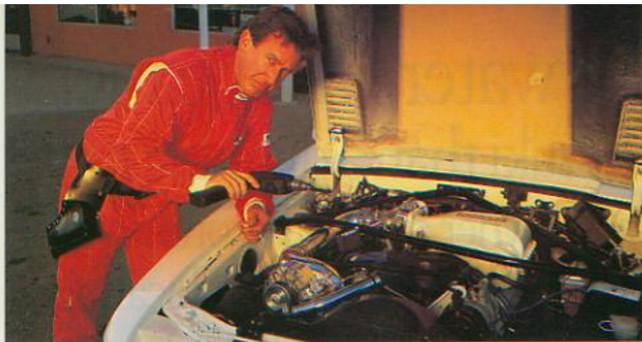
■ Drill out the jets? I don't think so, Tim. Mainly because there's no carburetor on this electronically fuel-injected, Vortech-supercharged Ford V-8.
