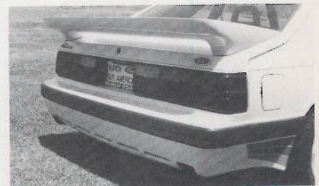
Saleen's lower rear valance reduces airstream updraft from under the car with accompanying dirt and moisture. Spoiler is bolted to rear deck to provide stabilizing downforce at speed.
